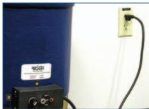
To use more than one Canister Heating Jacket in one 110 VAC outlet, plug the second Canister Heating Jacket into the plug outlet located on the control box of the first Canister Heating Jacket that is plugged into the 110 VAC outlet. In this manner, connect up to 5 Canister Heating Jackets in series, powered from one 110 VAC outlet.
