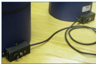
2. To install a canister, remove the Canister Heating Jacket lid and place the canister inside. Slide the cleaning pigtail or tubing through the hole in the Canister Heating Jacket lid and connect it to the valve on the canister, then place the lid on the Canister Heating Jacket. The lid should fit snugly onto the jacket.
