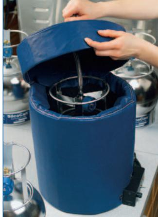
3. Turn on the power by selecting either the 75°C (canister with gauge) or 150°C (canister with valve only\*) temperature setting on the control panel on the Canister Heating Jacket.
